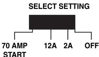
**Note:** For best results, charge the battery first for 10–20 minutes using the 10 A 12 V position before attempting to start the vehicle in the 70 AMP START position.
