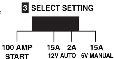
Engage the starter for 3–4 seconds; if engine fails to start, charge the battery using the 15 A 12 V position for another 10–20 minutes and attempt to start the engine again. Be aware that a typical starter on a vehicle may need 250–500 amps to start the engine.
