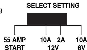
charge the battery using the 10 A 12 V position for another 10–20 minutes and attempt to start the engine again. Be aware that a typical starter on a vehicle may need 250–500 amps to start the engine.
