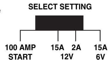
**Note:** For best results, charge the battery first for 10–20 minutes using the 15 A 12 V position before attempting to start the vehicle in the 100 AMP START position.
