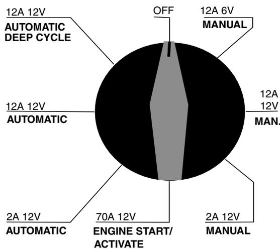
Rotate the selector switch to the 70A 12V position (70A 12V ENGINE START/ACTIVATE) for assistance in starting an engine with a weak battery. Plug the ac power cord into the wall outlet.
