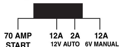
**Note:** For best results, charge the battery first for 10–20 minutes using the 12 A 12 V position before attempting to start the vehicle in the 70 AMP START position.
