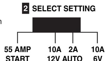
**Note:** For best results, charge the battery first for 10–20 minutes using the 10 A 12 V position before attempting to start the vehicle in the 55 AMP START position.
