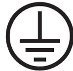
The frame of the welder must be grounded. A ground terminal marked with the symbol is located on the under panel for this purpose. See your local and national electrical codes for proper grounding methods.
